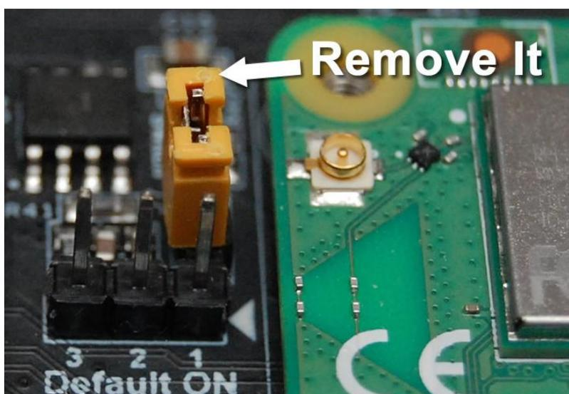
In addition, you will need to put a jumper cap on the "Default ON" jumper. This is to let you choose whether your PiGear Nano will automatically boot up when the power supply is connected. If you put the jumper cap on pin 3-2, it will not boot up until you tap the power button.
