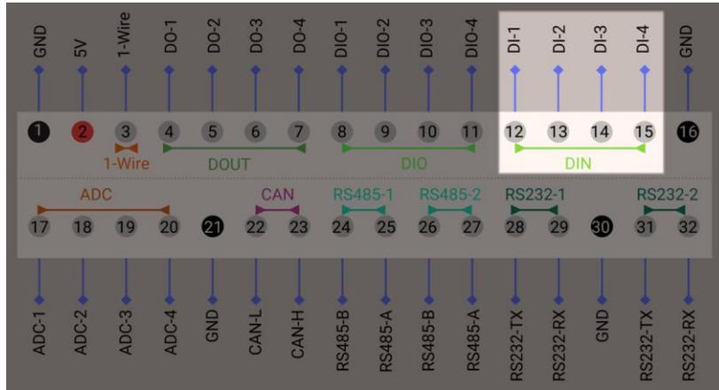
The four digital inputs are implemented by chip PCF8574, which talks to Raspberry Pi Compute Module 4 via the I2C-1 interface. Each digital input can bear up to 12V. Voltage below 0.5V is considered as LOW.
