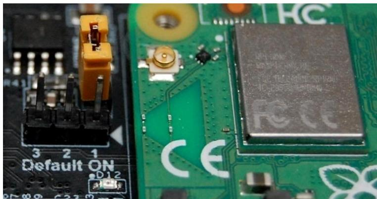
You will also need to short the "Disable eMMC Boot" jumper, so the eMMC on your Raspberry Pi CM4 will boot in USB mass storage mode, and you can flash the disk image into it.
