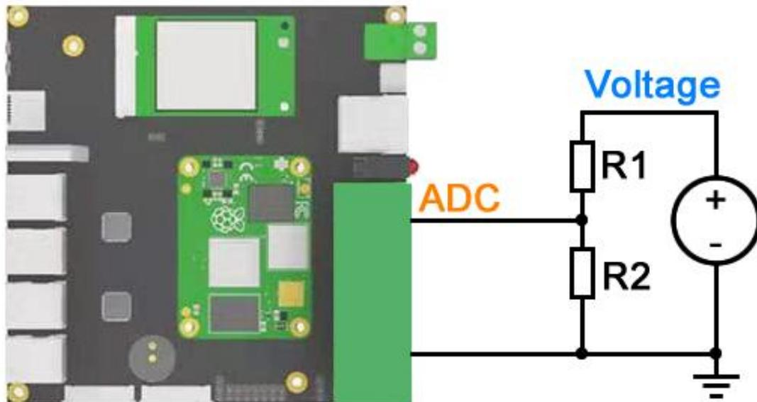
R1 and R2 should be properly chose so the actual voltage applies to ADC is no higher than 11.6V.
