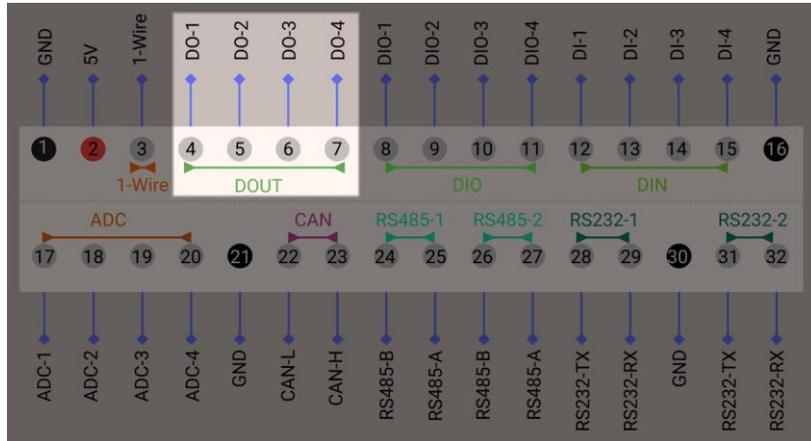
These 4 digital outputs are open drain outputs and they are driven by GPIO-11, GPIO-16, GPIO-17 and GPIO-22 in Raspberry Pi Compute Module 4 (please see table below).
