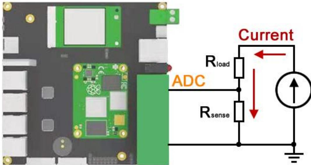
Usually  $R_{sense}$  is a rather small resistor. If  $R_{sense}$  is  $0.01 \Omega$ , and the voltage drops on  $R_{sense}$  is  $0.0125V$ , the current can be calculated like this:
