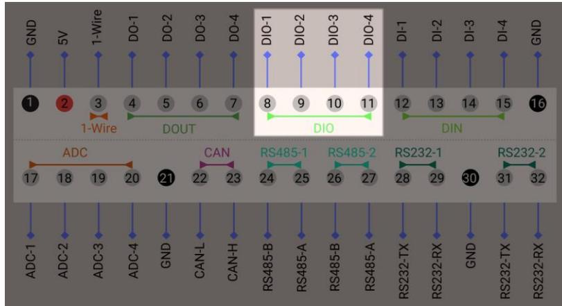
These four pins can be configured as either inputs or outputs. DIO-1 and DIO-2 are in one group, while DIO-3 and DIO-4 are in another group. The pins in the same group must be in the same input/output mode. Therefore, there are four possible configurations:
