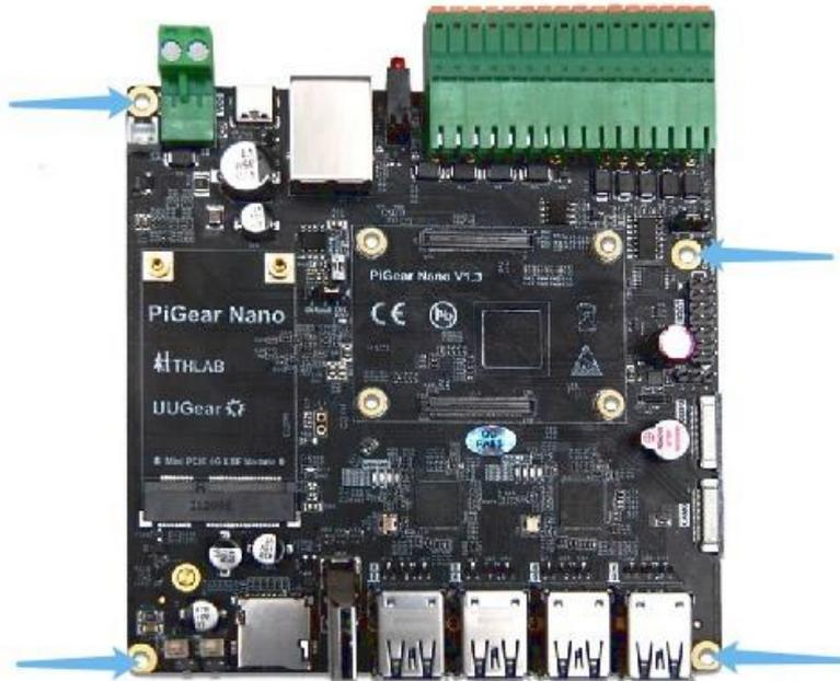
Connect Raspberry Pi Compute Module 4 to the board by simply aligning it with the two connectors on board (or alternatively you can align the CE marks on CM4 and the board), and then give it a good squeeze. It will crunch into place (and you can hear it).
