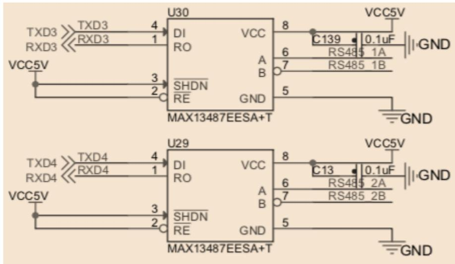
Both RS485 channels work in Half-Duplex mode, and they do not need additional I/O pin to control the transmitting direction.
