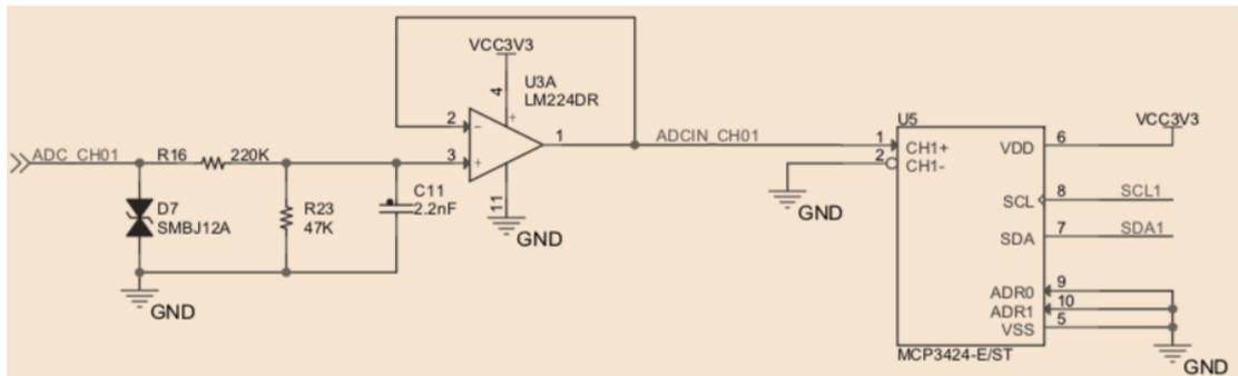
As shown in the schematic above, each channel has a voltage divider and a voltage follower before feeding to MCP3424. Because MCP3424 uses 2.048V internal voltage reference, each channel can directly measure up to 11.6V.
