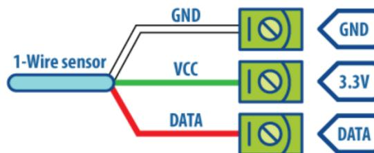
Some 1-wire device can be powered by the voltage on data line, and doesn't have the VCC wire.
