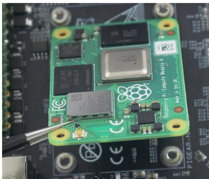
If you will use the device in a vibrating environment, you may want to secure your Raspberry Pi Compute Module 4 on the board with four M2.5 screws (not included in the package).
