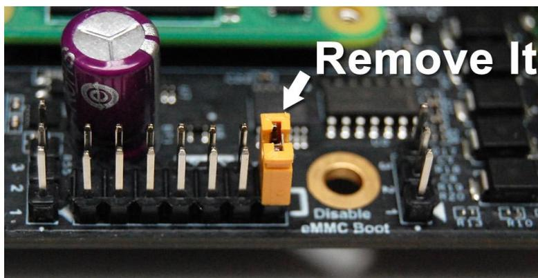
With the software installed, the e-latching power switch is supported on software level. However, you still need to remove the "bypass power switch" jumper cap, otherwise PiGear Nano cannot fully cut the power after system shutdown. If you do not want to use the e-latch power switch, you can keep this jumper cap in place.
